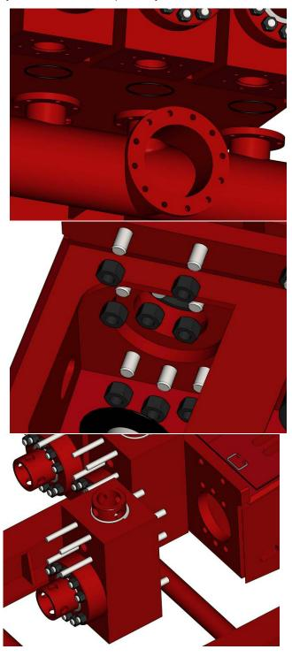
**2** Unbolt the fluid module from the frame.
