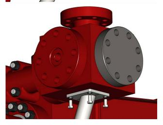
**4** Unbolt the discharge cross from its support and the discharge manifold, and remove.
