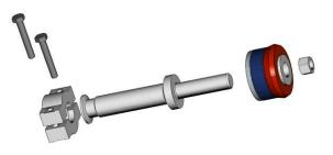
**2** Re-install the piston, ensuring that the seal remains properly aligned with the groove in the piston hub. Lock into position using the piston rod nut, and torque to 1,000 ft. lbs. torque (on a 1.5" piston rod nut).
