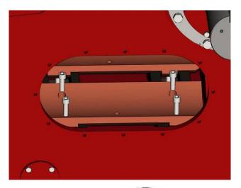
2 Install the outer race of the wrist pin bearing as per 5.3.5: Installing the Wrist Pin Bearing (page 95), then pack the wrist pin bearing rollers with grease to ensure that the rollers stay against the outer race during the wrist pin installation.
