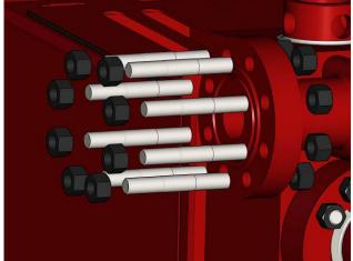
**2** Unbolt the Discharge Pulsation dampener from the Discharge cross and carefully lift from the power frame.
