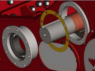
**9** Slide the shaft out of the pump frame. Since the bearings are carrier mounted, the shaft can be removed out of either side of the frame. However, be sure to note its original orientation, as it should be replaced facing the same direction.
