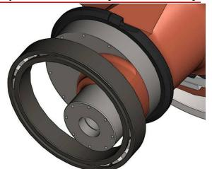
4 Install the inner retainer to lock the bearing into place.
