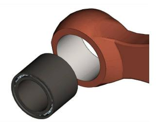
2 If the inner race of the wrist pin bearing needs to be replaced, it may be slipped off of the wrist pin by heating it with a torch. The bearing race should not have to be raised to over 200°F to press the wrist pin out of it.
