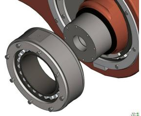
**5** Remove the main bearing oil seals from the crankshaft.
