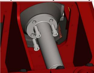
**7** Replace the diaphragm plates and bolt into position in the power frame.
