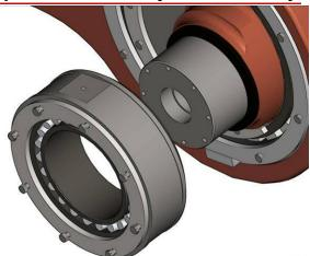
**5** Install the inner retainer of the main bearing and bolt all retainers in accordance with the Torque Chart (page 55).
