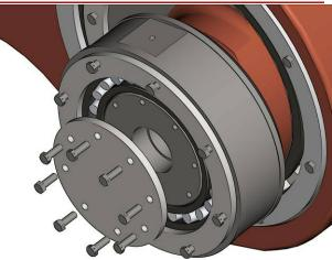
4 Slide the main bearing and shims free of the crankshaft.
