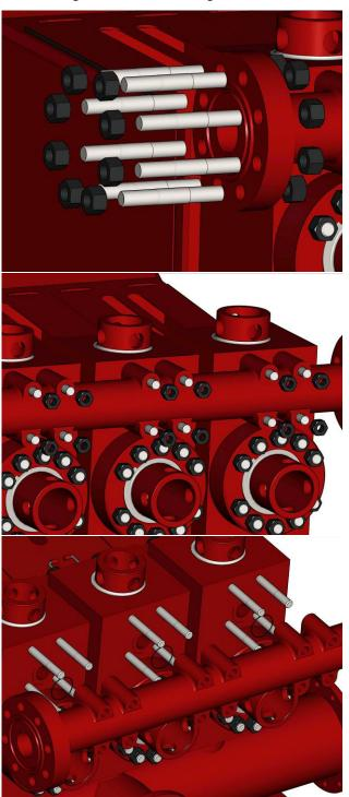
2 Remove the nuts connecting each of the discharge modules to the discharge manifold.
