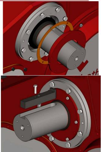
7 Once all maintenance is complete, reconnect the oil lube lines and pressurize the system. Reattach key as required.
