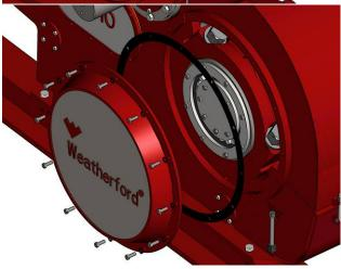
4 Replace the rear cover of the power frame and secure into place.
