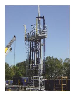
The 340K is a stand-alone snubbing unit designed and custom built to perform live or dead well interventions. It has the capabilities to run tubing from 2  $\frac{3}{8}$ " to 9  $\frac{5}{8}$ " and has 22,000 ft/lbs. rotary that allows it to take on tasks unheard of in the snubbing industry such as drilling, milling out windows for side tracks and side tracking.
