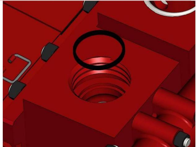
**8** Coat the bottom seating surface and outside of the valve covers with grease and screw into place over the valve bores.
